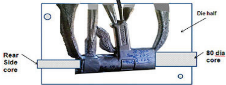
In correct orientation of the casting in the existing die
